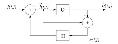
Figure 7: Block diagram of the error diffusion method.
